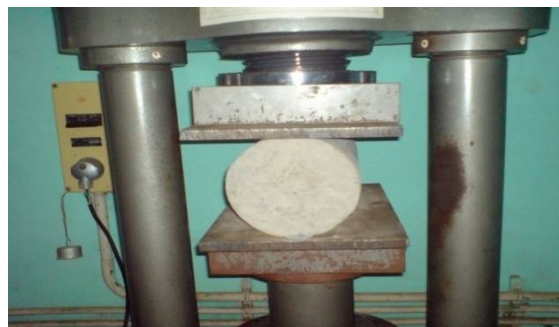
Figure 4.2 Split Tensile Test
