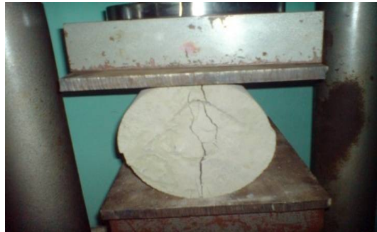
Figure 4.3 Failure of Cylinder
